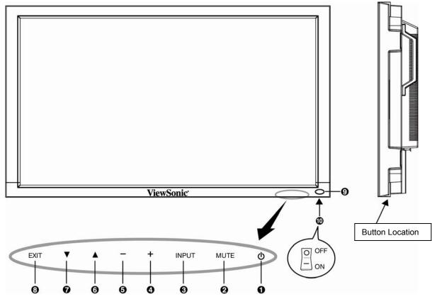
**OPOWER button (O) -** Switches the power on/off.
